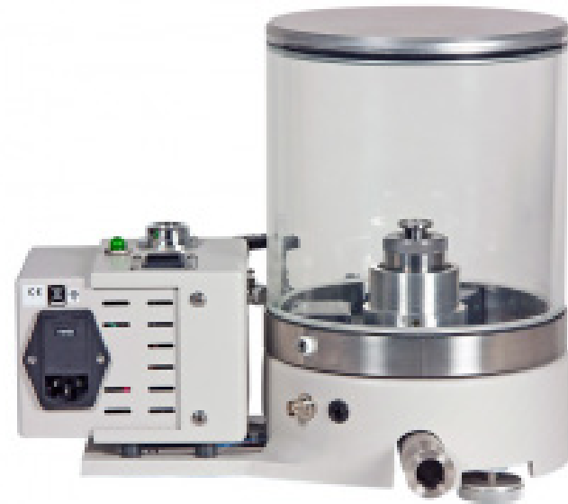
Figure 1: Ruska Pressure Balance with Weight Stack
